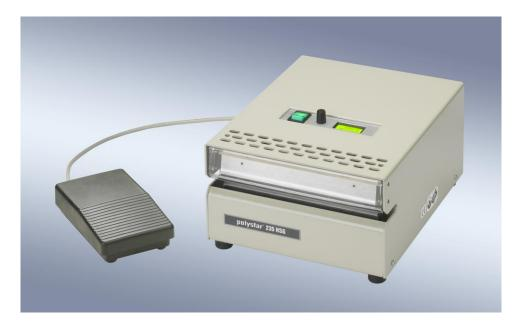
Easy heat sealing with foot pedal: For all sealable materials (e.g. aluminium or paper foils, cellophane, etc.) up to seal length of max. 235 mm. Of course, this heat sealer is GS-approved! Equipped with incremental encoder for setting of temperature and sealing time. Parameter specifications via display. After successful setting of parameters and preheating time just place the sealing material between the heating elements. Then, simply press the foot pedal for starting your work.
